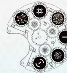
1 Rotating Gobo Wheel: 6 interchangeable metal gobos + white Gobo Ø25.9mm, image Ø13mm Bi-directional scrolling at variable speed Gobo shake effect at variable speed Gobo indexable
